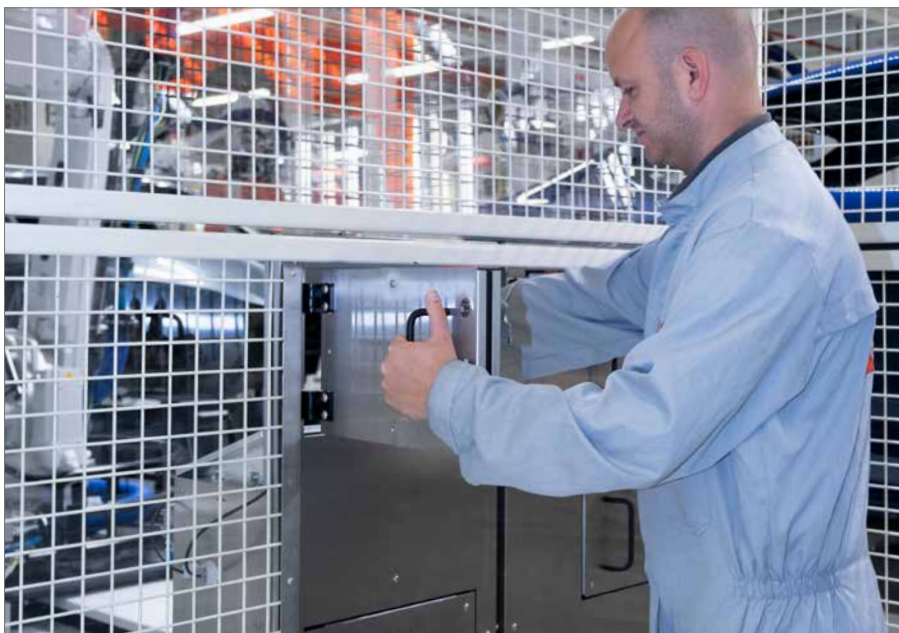
Eight polishing pad magazines for quick change, refillable during operation.
