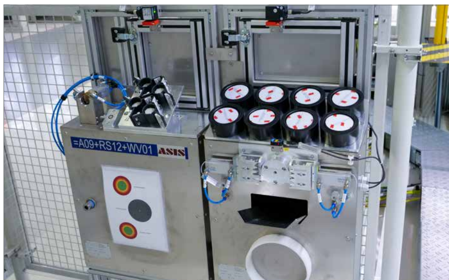
Four interchangeable magazines for quick abrasive change
