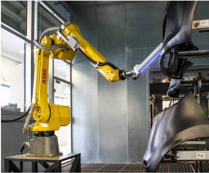
Fig. 2: Robot-controlled flame treatment of three-dimensional plastic parts
